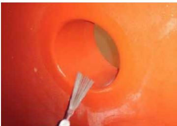
This Sulphuric Acid storage tank at Monómeros Colombo Venezolanos uses ChemLine® 784/32 coating for superior corrosion protection. Here, prior to being put into service, the coating in the tank is spark tested as part of a thorough inspection process.
