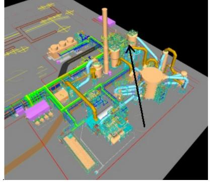
The 3D models enabled PCS to focus in on how the detailed design was progressing and to see items like valve accessibility and platform placement.
