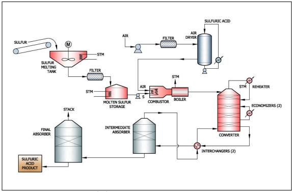
Sulfuric Acid Process Flow Diagram
