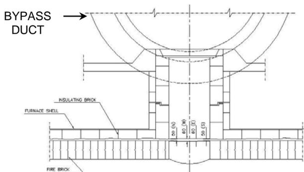
**Fig 2 Sulphur Furnace – Gap in Bricklining**
