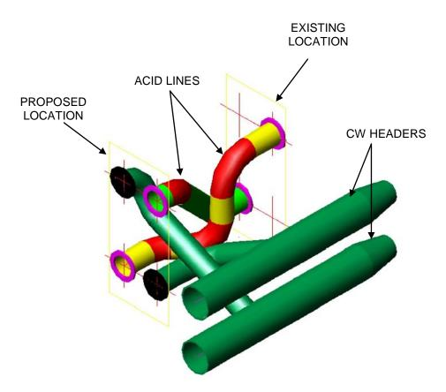
Fig 5 Scheme for interchanging Acid ports in Acid coolers
