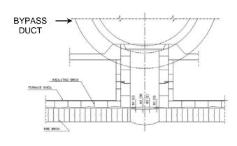
Fig 2 Sulphur Furnace – Gap in Bricklining
