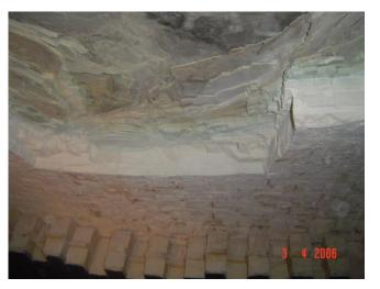
Fig 3 Sulphur Furnace – Accumulated Sludge
