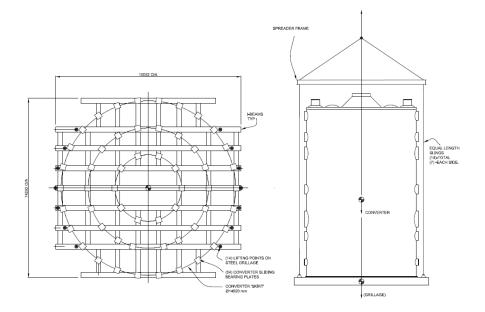
In practise, however, this turned out to be an impractical solution, so Bateman Engineering designed a new lifting arrangement for each converter, which could now be fully utilised in Durban South Africa, at the Madagascan port of Tamatave and on site.
