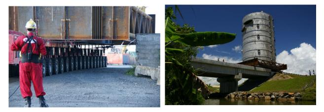
The SPMTs, which are remote controlled by a highly skilled operator, were free issued to Bateman Engineering by the Client. Remarkably this massive vehicle was ideal for this application as it's load bed remained level with the wheel heights varying to accommodate any undulations in the road surface, thus keeping the load stable at all times. Figure 13 : SMPT wheel articulation
